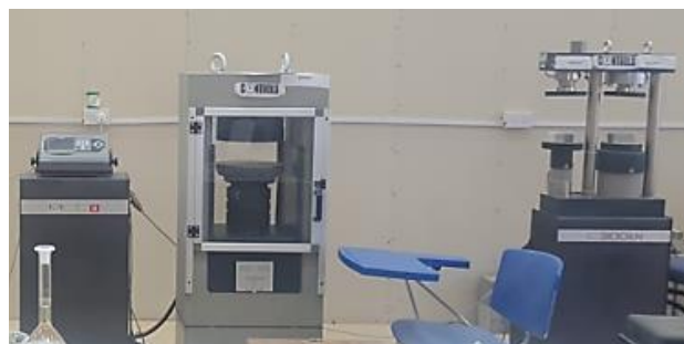
Compression and Flexural testing Machine for Cement and Concrete (3000 kN)
