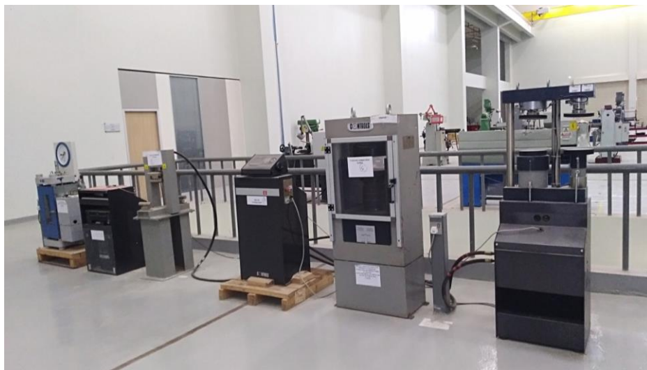
Fig.: Compression and Flexural testing Machine for Cement and Concrete (3000 kN) for testing Direct Compressive Strength of Cement Mortar, concrete cubes and Cylinders.
