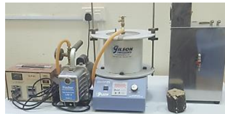
Gilson Vibro-Deaerator (Rice) with Vacuum Pycnometer, 2,000g
