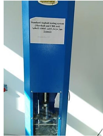
Standard Asphalt Testing Device-compactor (Marshall and CBR)
