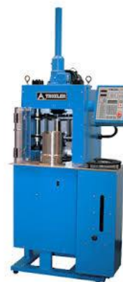
Troxler Superpave Gyratory Compactor, SHRP Package
