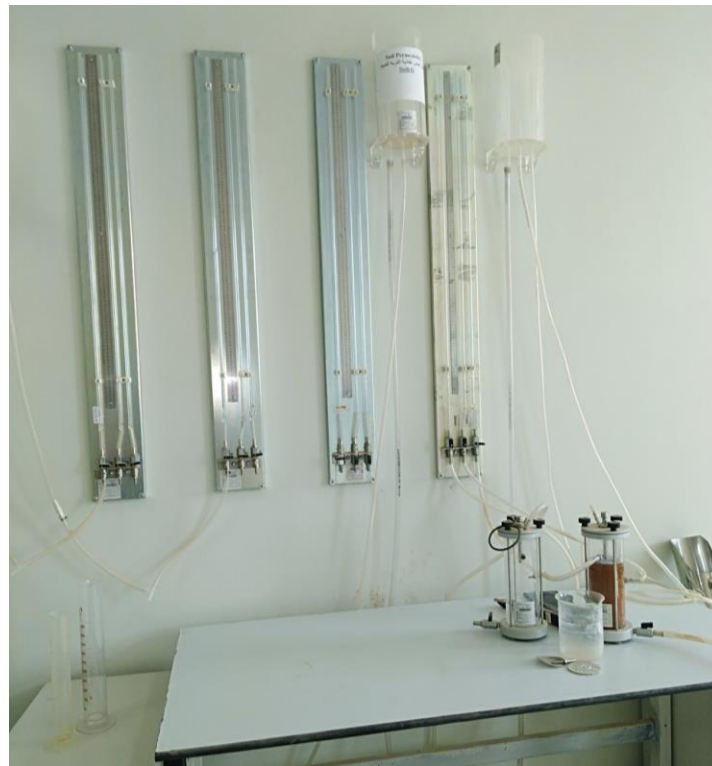
Fig.: Constant head and Falling Head Permeameter device for Permeability Test for Granular Soil
