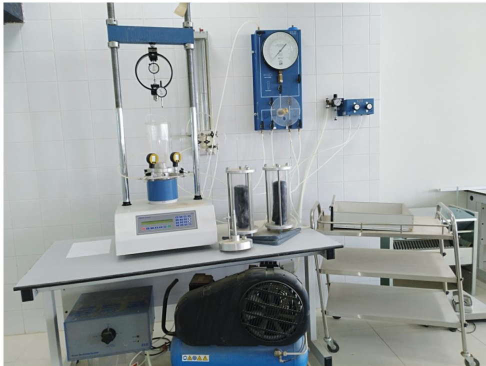
Fig.: Tri-axial compression machine used for Tri-axial Compression Test
