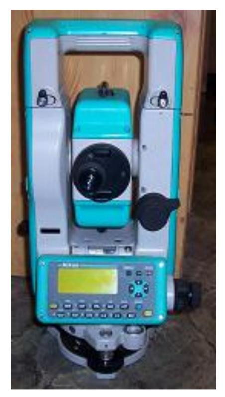
Figure 2: Example of Digital Theodolite
