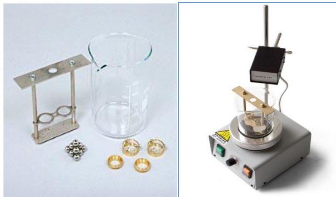
Figure 8.1 Ring and Ball apparatus
