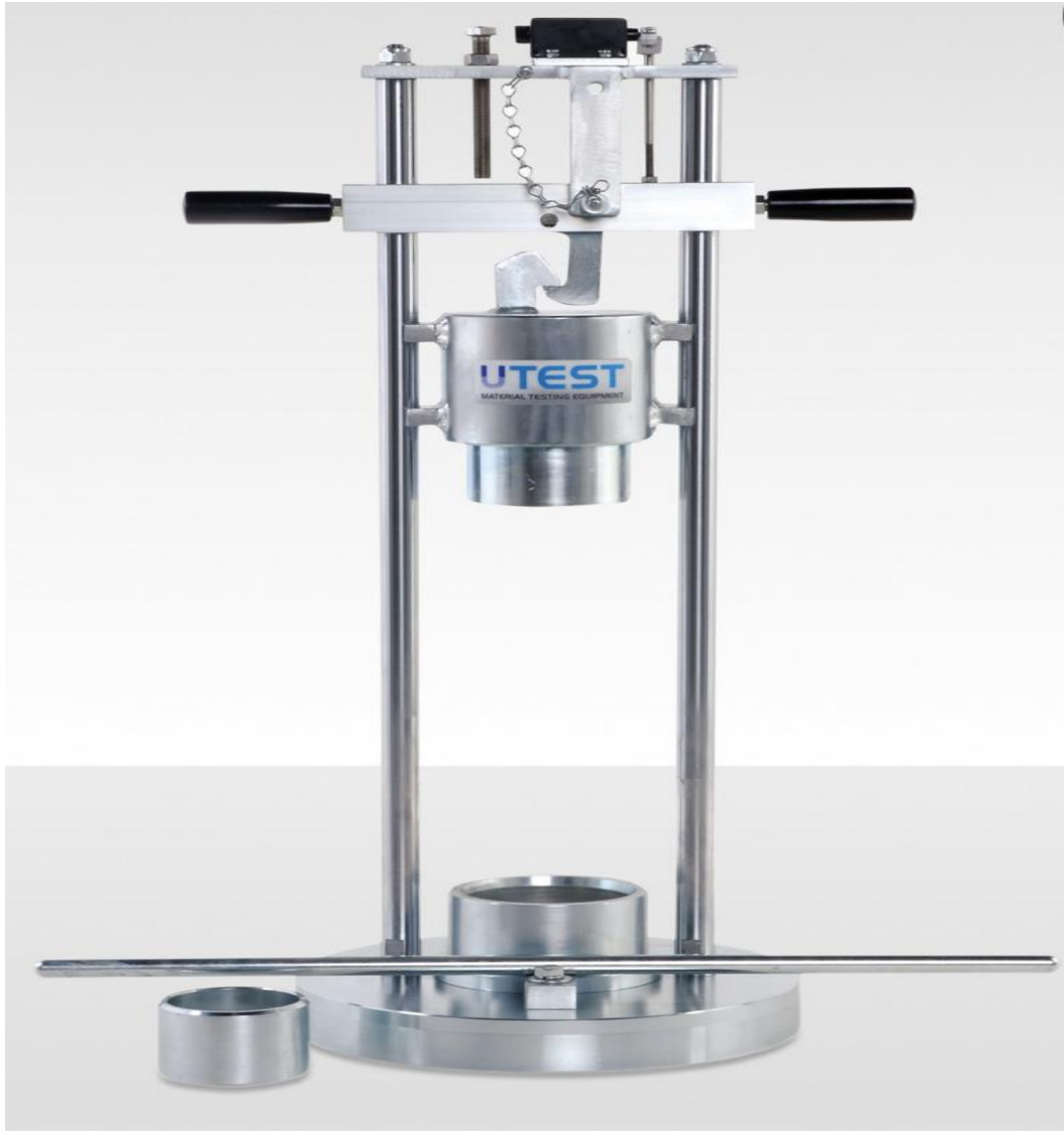
Figure 4.1 Aggregate Impact Test machine
